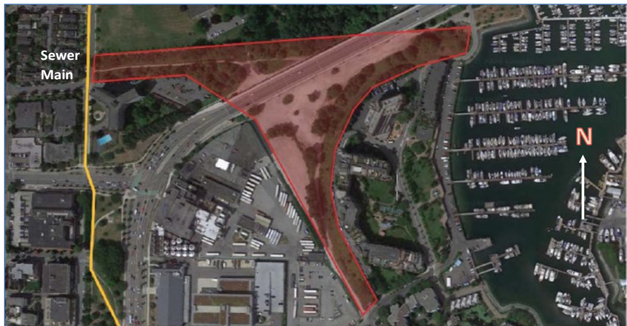
Figure 4: Sewer Heat Recovery tie-in location
